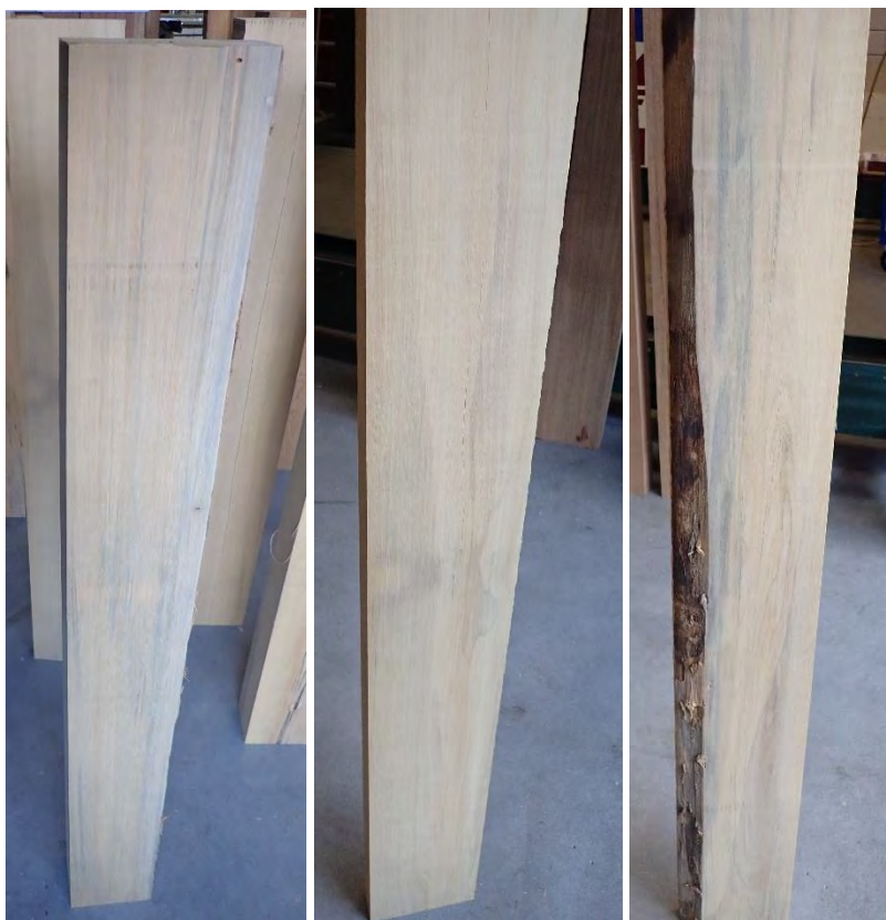
Figure 3.5.1 Kimboto planks sawn and planed, blue stain and wane
