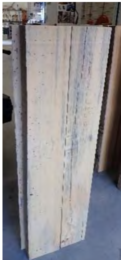
Boreholes with blue stain (rot)
