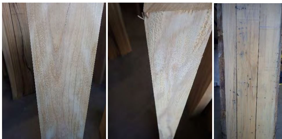
Figure 3.2.1 Bostamarinde heartwood, reaction wood and sapwood
